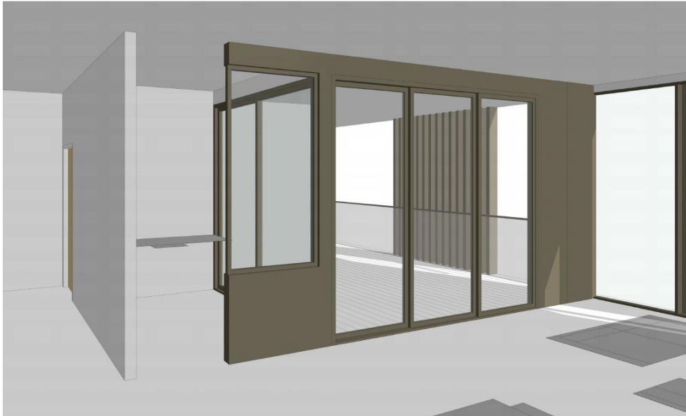
Figure 8: Diagram showing the short wall facing the hall way to be deleted and replaced with a half panel with glazing – applicable for studies in Unit types 2B.04, 2B.07C, 2B.10, and 2B.11
